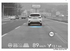
The Head-Up Display is an optional feature that allows the driver to view information projected onto a transparent screen while still keeping your eyes safely on the road ahead while driving.
