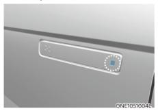
Push the button on the front outside door handle (the engraved part) while carrying the Smart Key with you, all doors will lock.
