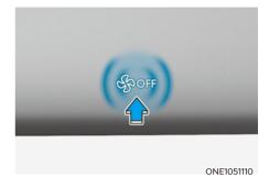
Touch the OFF icon to turn the climate control system off. You can still operate mode selection and air intake control as long as the Start/Stop button is in the ON position.
