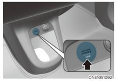
You can use an USB cable to connect audio devices to the vehicle USB port.
