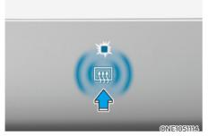
The defroster heats the window to remove frost, fog and thin ice from the interior and exterior of the rear window, while the vehicle is running.
