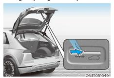
To unlock and open the tailgate manually from inside the luggage compartment, perform the following procedure:
