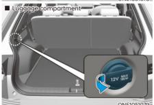
The power outlet is designed to provide power for mobile telephones or other devices designed to operate with vehicle electrical systems. The devices should draw less than 180 watts with the vehicle running.
