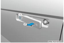
Push the button on the front outside door handle (the engraved part) while carrying the Smart Key with you, all doors will unlock.
