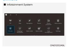
To view the climate information screen, select Climate in the main infotainment screen when the vehicle is ON.
