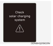
When the solar roof controller is not working properly, the 'Check solar charging system' warning message will appear on the cluster. We recommend to take your vehicle to an authorized HYUNDAI dealer and have the system checked.
