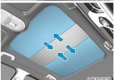
The power sunshade can only be operated when Start/Stop button is in the ON or START position.
