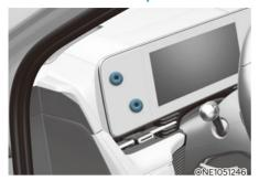
The cluster fascia side panel is a pad to attach light items such as parking tickets, receipts, etc., using its magnetic surface.
