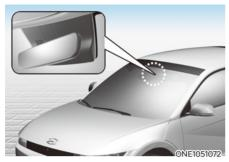
The rain sensor located on the upper end of the windshield glass senses the amount of rainfall and controls the wiping cycle for the proper interval.
