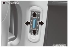
The instrument panel vent air flow can be directed up/down or left/right using the vent adjustment lever.
