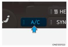
Touch the CLIMATE icon in the climate control panel. The climate information screen will appear on the infotainment screen. Touch the A/C icon in the infotainment screen to turn the air conditioning on (indicator light ON) and off.
