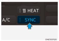
Adjusting the temperature and air flow direction equally
