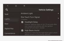
With the Start/Stop button in the ON position, select 'Lights → High Beam Assist (or HBA (High Beam Assist))' from the Settings menu to turn on High Beam Assist and deselect to turn off the function.
