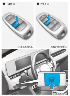
Power tailgate open/close button (Smart key, Instrument panel)
