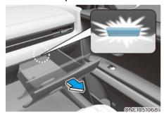
The glove box lamp turns on for about 20 minutes when the glove box is opened.
