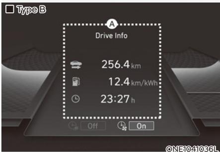
Driving Assist, Turn by Turn, Utility view modes are displayed in the center (A) of the instrument cluster.
