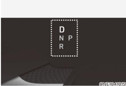
The indicator displays which gear is selected.
