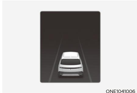
The status of Manual Speed Limit Assist, Smart Cruise Control, Lane Following Assist, Highway Driving Assist, etc., is displayed when Driving Assist view is selected.
