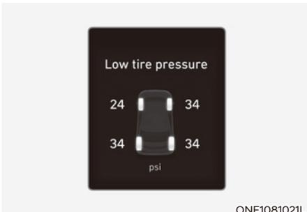
This warning message is displayed if the tire pressure is low. The corresponding tire on the vehicle will be illuminated.
