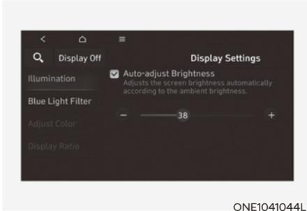
The brightness of the instrument panel can also be adjusted from the infotainment system screen. When Start/Stop button is in the ON position, select 'Settings → Display → Illumination'.
