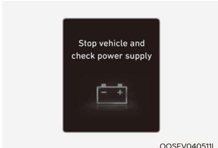
This warning message is displayed when a failure occurs in the power supply system.
