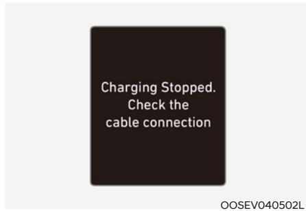
This warning message is displayed when charging is stopped because the charging connector is not correctly connected to the charging inlet
