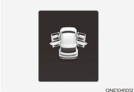
This warning is displayed if any door or hood or tailgate is left open. The warning will indicate which door is open in the display.
