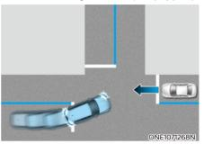
Junction Turning function will help avoid a collision with an oncoming vehicle in an adjacent lane when turning left (lefthand drive) or right (right-hand drive) at a crossroad with the turn signal on by applying emergency braking.
