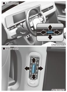
The instrument panel vent air flow can be directed up/down or left/right using the vent adjustment lever.
