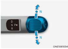
To shift the gear to N (Neutral), rotate the rotary gear shift dial to N (Neutral) while depressing the brake pedal.
