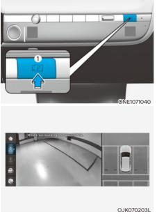
Surround View Monitor can assist in parking by allowing the driver to see around the vehicle.
