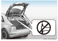
Do not grab or hold on to the tailgate support struts at any time. Damage to the tailgate support struts could result. Deformation of the tailgate support struts may cause vehicle damage and personal injury may occur.
