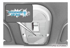
To reactivate the passenger's front air bag:
