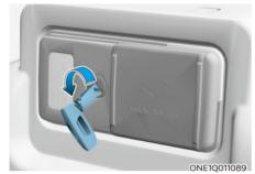
Use the smart key to unlock the power outlet cover.
