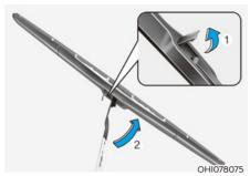
1. Lift up the wiper blade clip (1). Then lift up the wiper blade.
