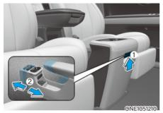
To slide the console (2) forward/ backward, pressing the handle (1) and pull or push the console to the desired position.
