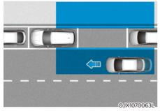
After the vehicle stops, when an approaching vehicle from the rear area is detected as soon as a passenger opens a door, Safe Exit Warning will warn the driver with a warning message and an audible warning to help prevent a collision.
