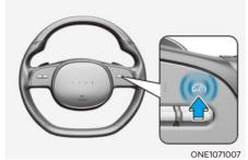
Press the Driving Assist (C) button to turn Cruise Control off. The Cruise (CRUISE) indicator will go off.
