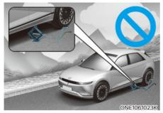
Never start or run the vehicle while an 4WD vehicle is raised on a jack. The vehicle can slip or roll off of a jack causing serious injury or death to you or those nearby.
