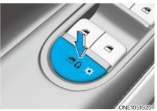
When the electronic child safety lock button is pressed and the indicator light on the button illuminates, the rear doors cannot be opened from inside the vehicle.
