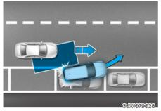
When you are driving forward out of a parking space, if Blind-Spot Collision-Avoidance Assist judges that there is a collision risk with an approaching vehicle in the blind spot, it will help avoid collision by applying the brake.
