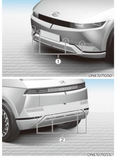
[1] : Front ultrasonic sensors,[2] : Rear ultrasonic sensors
