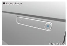
To unlock your vehicle using the door handle button or the Smart Key:
