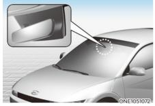
The rain sensor located on the upper end of the windshield glass senses the amount of rainfall and controls the wiping cycle for the proper interval.
