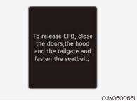
To release EPB, close the doors, hood and tailgate and fasten the seatbelt
