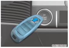
If the smart key battery is weak or the smart key does not work correctly, you can start the vehicle by pressing the Start/Stop button with the smart key in the direction of the picture above.
