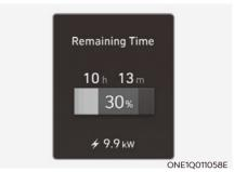
10.After charging has started, the estimated charging time is displayed on the instrument cluster for about 1 minute.
