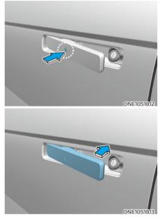
When all doors are closed, touch the touch sensor on the front outside door handle (the engraved part) while carrying the Smart Key with you, outside door handle will return and doors will be locked.
