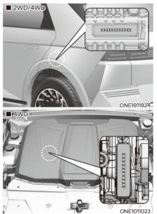
The motor numbers can be checked at the bottom of the vehicle.
