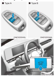
Power tailgate open/close button (Smart key, Instrument panel)
