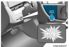
With the driver's door and hood closed, depress the brake pedal and then press the AUTO HOLD switch. The white AUTO HOLD indicator will come on and the system will be in the standby position.
