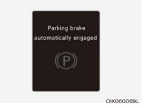
Parking brake automatically engaged When EPB is applied while Auto Hold is activated, a warning will sound and a message will appear.
