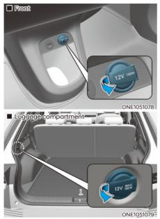
The power outlet is designed to provide power for mobile telephones or other devices designed to operate with vehicle electrical systems. The devices should draw less than 180 watts with the vehicle running.
