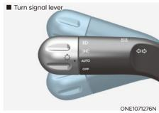
Highway Lane Change Assist function will operate, when you push the turn signal lever up or down to the A or B position while the function is in the ready state (**† t** indicator is green), and all of the following conditions are satisfied:
