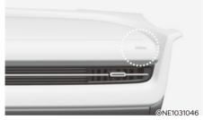
Your vehicle is equipped with a Supplemental Restraint System (SRS) and lap/shoulder belts at both the driver and passenger seating positions. The SRS consists of air bags which are located in the center of the steering wheel and the passenger's side front panel pad above the glove box.
