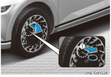
For 20 inches wheel, take out the remover tool (1) in the Tire Mobility Kit. Insert the tool to the hole and pull out the wheel cover.
