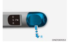
To shift the gear to R (Reverse), rotate the rotary gear shift dial to R (Reverse) while depressing the brake pedal.
