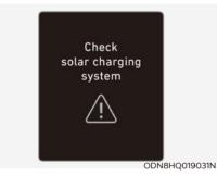
When the solar roof controller is not working properly, the 'Check solar charging system' warning message will appear on the cluster. We recommend to take your vehicle to an authorized HYUNDAI dealer and have the system checked.
