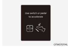
In traffic, your vehicle will stop if the vehicle ahead of you stops. Also, if the vehicle ahead of you starts moving, your vehicle will start as well. In addition, after the vehicle has stopped and a certain time have passed, the 'Use switch or pedal to accelerate' message will appear on the cluster. Depress the accelerator pedal or push the + switch, - switch or II' switch to start driving.
