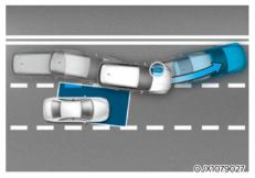
When changing lanes by detecting the lane ahead, if Blind-Spot Collision-Avoidance Assist judges that there is a collision risk with an approaching vehicle in the blind spot, it will help avoid collision by applying the brake.
