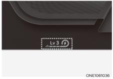
The regenerative brake indicates the level of the regenerative braking that you set. And it also indicates Smart regenerative system's operation status.
