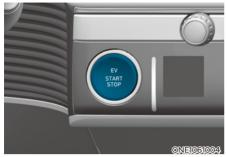
Whenever the front door is opened, the Start/Stop button will illuminate and will go off 30 seconds after the door is closed.
