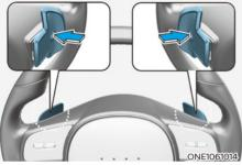
The paddle shifter is used to adjust the regenerative braking level from 0 to 3 during decelerating.
