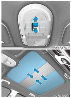
The power sunshade can only be operated when Start/Stop button is in the ON or START position.
