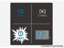
Plugged into vehicle (POWER Green ON, FAULT Red Blink)
