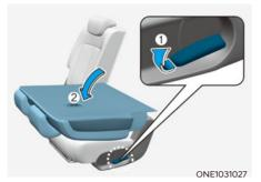
4. Pull up the seatback folding lever (1), then fold the seat (2) toward the front of the vehicle. When you return the seatback to its upright position, always be sure it has locked into position by pushing on the top of the seatback.
