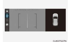
When you touch the **s**icon, the top view is displayed on the screen and shows the distance from the vehicle in the back of your vehicle while parking.
