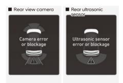
ONE1071056L ONE1071106L The 'Camera error or blockage' or 'Ultrasonic sensor error or blockage' warning message will appear on the cluster if the following situations occur:
