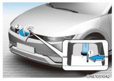
3. Go to the front of the vehicle, raise the hood slightly, push to the left the secondary latch (1) inside of the hood center and lift the hood (2).
