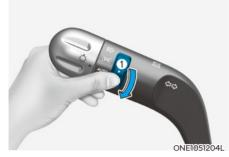
To turn on the rear fog lamp: Position the headlamp switch in the headlamp position, and then turn the headlamp switch (1) to the rear fog lamp position.
