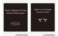
When Highway Driving Assist or Highway Lane Change function is not working properly, the 'Check Highway Driving Assist (HDA) system' or 'Check Lane Change Assist function' warning message will appear, and the  $\triangle$  warning light will illuminate on the cluster. We recommend that the vehicle be inspected by an authorized HYUNDAI dealer.
