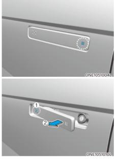
Push the button on the front outside door handle (the engraved part) while carrying the Smart Key with you, all doors will unlock.
