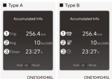
This display shows the accumulated trip distance (1), the average energy consumption (2), and the total driving time (3).
