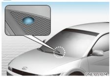
Never place anything near the ambient light/solar sensor to ensure better control of the heating and cooling system.
