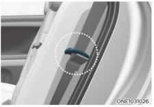
3. Route the seat belt webbing to the outward of the rear seat to prevent the belts from being trapped behind or under the seats.
