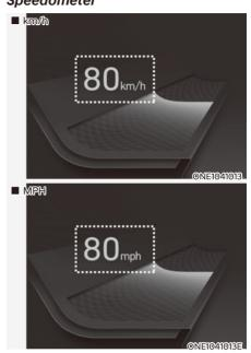
The speedometer indicates the speed of the vehicle and is calibrated in kilometers per hour (km/h) and/or miles per hour (MPH).
