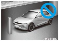
Remote Smart Parking Assist performance may reduce or collision with an obstacle may occur when there is a narrow object, circular pillar, square pillar, or a pillar surrounded by objects such as a fire extinguisher, etc., near the parking space. The driver should park the vehicle manually.
