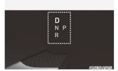
The indicator displays which gear is selected.
