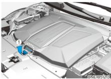
2. Lift up the front trunk cover while depressing the front trunk lever (1).
