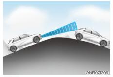
When coasting on an uphill or downhill, the system may not detect the vehicle in your lane and the regenerative braking level will reduce automatically, making you feel that the vehicle is accelerating.
