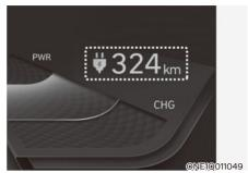
The distance to empty is displayed differently according to the selected drive mode in the Drive Mode Integrated Control System.
