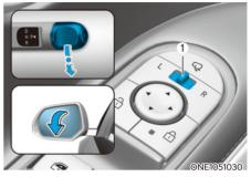
When the gear is shifted to the R (Reverse) position, the outside rearview lever(s) will rotate downwards to aid with driving in reverse.
