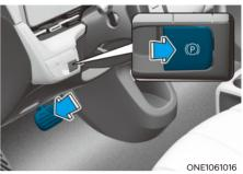
To release EPB (Electronic Parking Brake):
