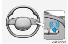
To turn off Smart Cruise Control Press the Driving Assist (උත) button to turn Smart Cruise Control off.
