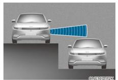
Blind-Spot Collision-Avoidance Assist may not operate properly when driving where the heights of the lanes are different. The function may not detect the vehicle on a road with different lane heights (underpass joining section, grade separated intersections, etc.).
