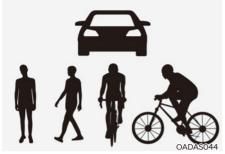
The illustration above shows the image the front view camera and front radar will detect as a vehicle, pedestrian and cyclist.
