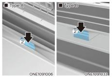
3. Remove the cover by pulling the front trunk handle (2).
