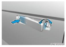
Press the front part (1) of the door handle to pull out the rear part of the door handle. While keep pressing the front part of the door handle, insert the mechanical key to the lock.
