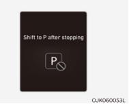
This message is displayed when the gear is shifted to P (Park) while the vehicle is moving.
