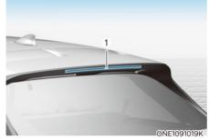
If the LED lamp (1) does not operate, we recommend that the system be inspected by an authorized HYUNDAI dealer.
