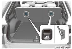
Top-tether anchorages for Child Restraint Systems are located on the rear of the seatbacks.
