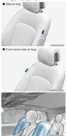
Your vehicle is equipped with a side air bag in each front seat. The purpose of the air bag is to provide the vehicle's additional protection than that offered by the seat belt alone.
