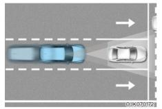
Forward Collision-Avoidance Assist is designed to help detect and monitor the vehicle ahead or help detect a pedestrian or cyclist in the roadway and warn the driver that a collision is imminent with a warning message and an audible warning, apply emergency braking.
