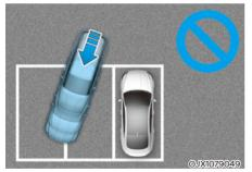
If Remote Smart Parking Assist is used, when parking in a parking space with a vehicle only on one side, your vehicle may cross the parking line to avoid the parked vehicle. Parking diagonal
