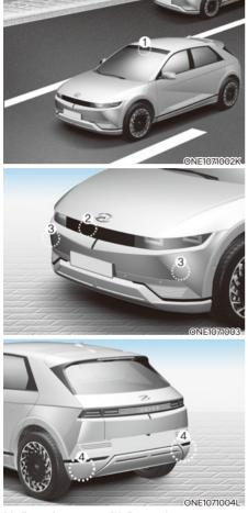
[1] : Front view camera, [2]: Front radar, [3] : Front corner radar (if equipped),
