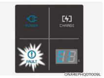
Before plugging charging connector into vehicle (POWER Green ON, FAULT Red blink)
