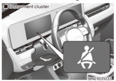
As a reminder to the driver, the driver's seat belt warning lights will illuminate for approximately 6 seconds each time the START/STOP button is in the ON position regardless of belt fastening. If the seatbelt is not fastened, the warning chime will sound for about 6 seconds.
