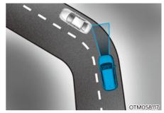
When coasting on the curve, the system may not detect the vehicle in your lane and the regenerative braking level will reduce automatically, making you feel that the vehicle is accelerating.
