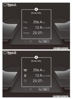
Driving Assist, Turn by Turn, Utility view modes are displayed in the center (A) of the instrument cluster.
